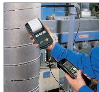
Check volume flow via thermal probe, e.g. in a ventilation duct with printout of data
